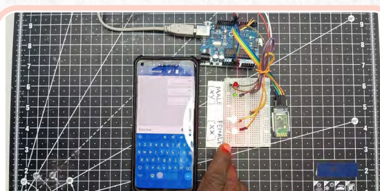
Sex Determination Model using Arduino, Bluetooth module, PictoBlox, and Dabble Application
