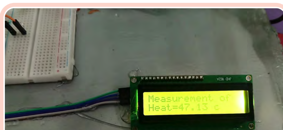
Temperature rises after the chemical reaction indicating the heat generation.
