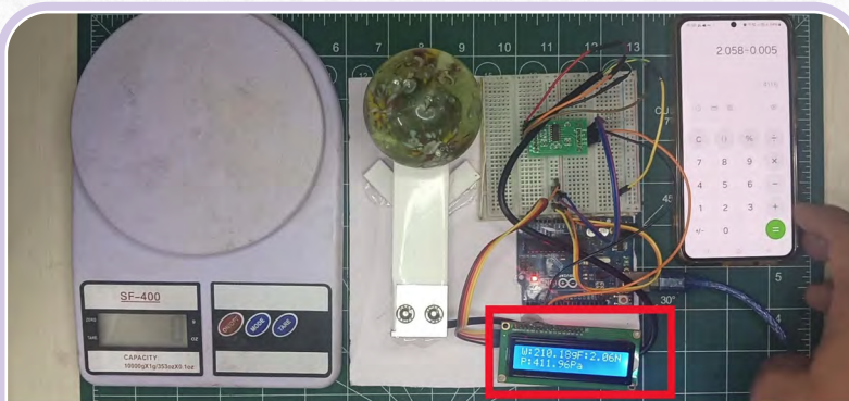
Measurement of Mass, Force and Pressure using Load Cell and Arduino Uno
