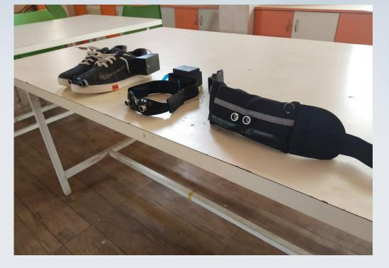
in this module. This assembly would be connected with Wi-Fi, working with a 3.3 V supply. So, when an object comes in front of the sensor, the ultrasonic sound waves would strike the object and trigger a signal to the Arduino board, which in turn would command the buzzer and vibrator to buzz or vibrate respectively and sound an alert to the user.
