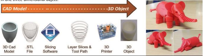
Technology used in ATLs: Fused Deposition Modelling (FDM) Technology
